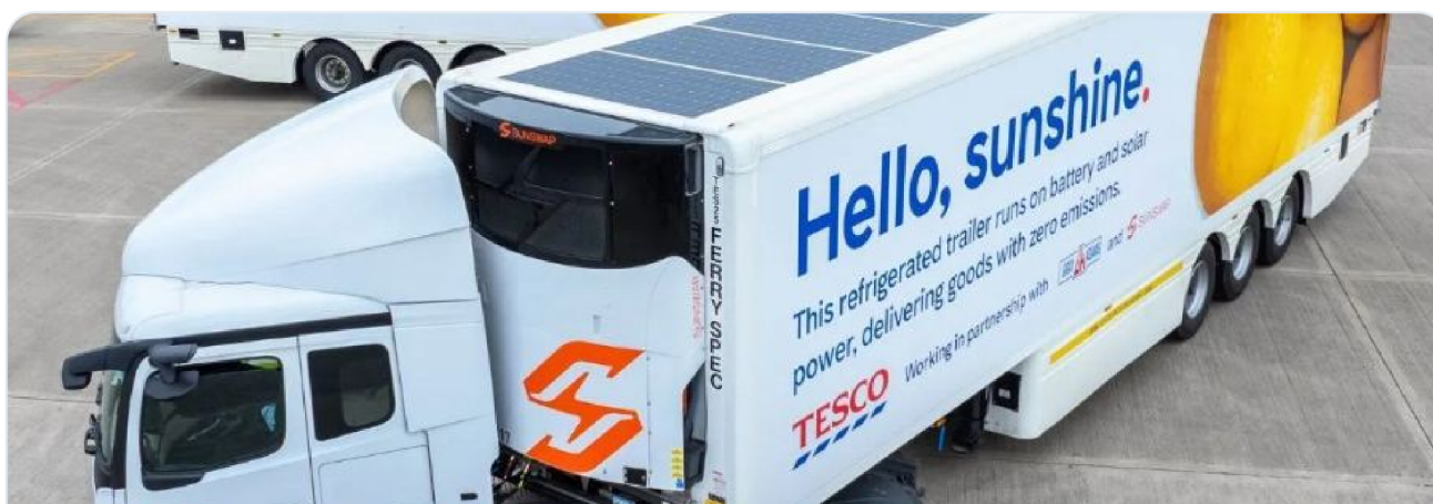
Sunswap's solar- and battery-powered refrigerated trailers in service with Tesco - delivering chilled goods with zero emissions at the point of use.
